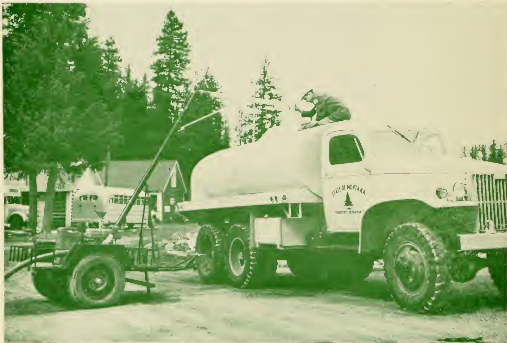
The tanker shown is military excess equipment redesigned and remodeled by State Forestry personnel to fill in gaps in needed fire equipment. The trailer, built in the Stillwater State Forest shop, carries a military excess pumper unit. This unit refills tanker in less than 5 minutes from any available water supply. In the background are 2 buses, also military excess equipment, used to haul fire fighters or to serve as mobile lookouts.
